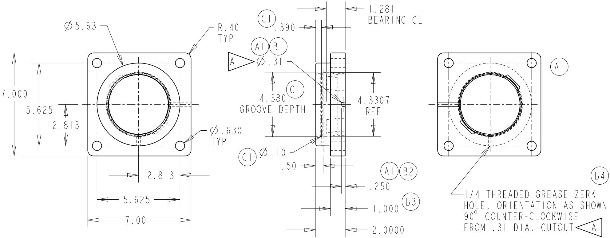
NOTE: MACHINE BEARING SURFACE OD FOR 110 MM INSERT BEARING
