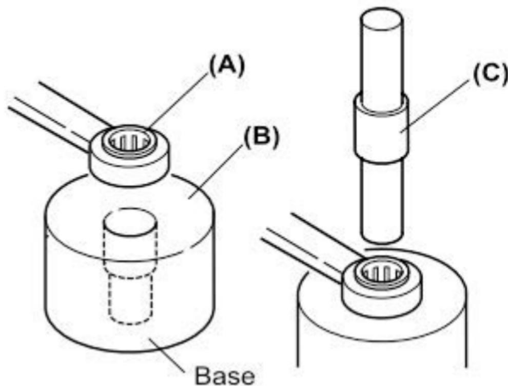
Tool to replace the needle bearing on small end of the connecting rod.
